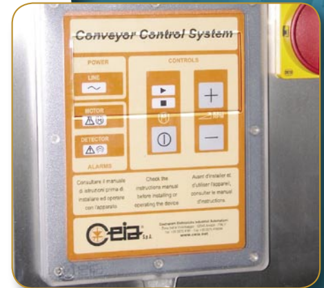
CONTROL PANEL ON CONVEYOR CONTROL SYSTEM
