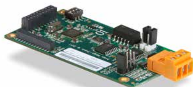
Analog Output Card 0-10 VDC and 4-20 mA.
