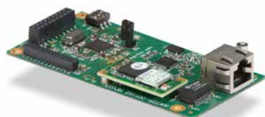
Wireless Ethernet Internal Card 802.11b/g Wireless
