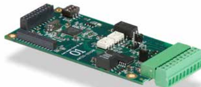
Current Loop Card Current Loop/RS485/RS422.
